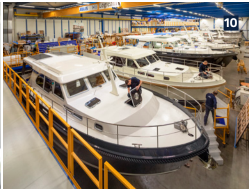
9. Logicam I production line (30'-35' Grand Sturdy & SL, engine room/interior)
